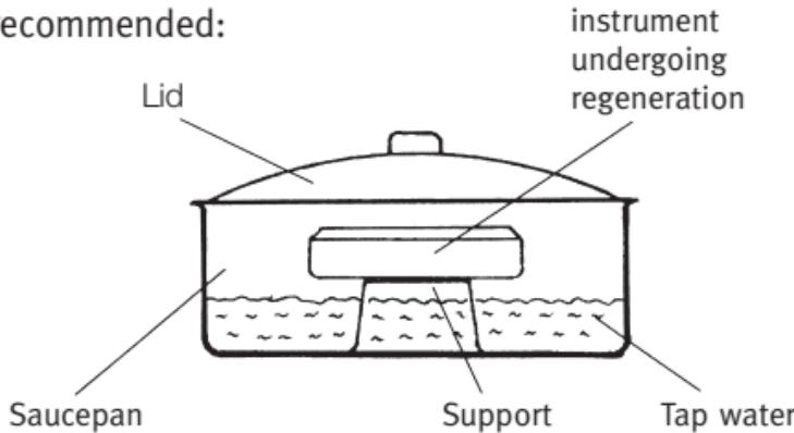
Fill a sizeable saucepan a quarter full of tap water (see illustration) and place the Hygrometer (or combined Thermo/Hygro) to be adjusted, on a stand as shown. It is important that the instrument does not drop into the water. It might be prudent to secure the instrument on to the stand (rubber band etc.). Finally, place a well-
