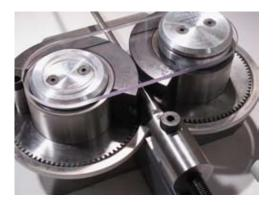
5 When the roller dies rotate, they will press the terminal shank onto the wire rope.
