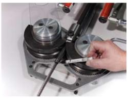
**3** Apply just enough hydraulic pressure so that the roller dies holds the terminal firmly. Then mark and insert the cable into the bottom of the terminal throat.
