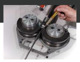
Choose the pair of roller dies that corresponds to the cable diameter, and slip them onto the cogwheel synchronizing pins. The arrows on the dies should always be in the swaging direction.
