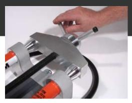
2 Attach the terminal to the attachment fixture on the drawbar, and adjust the length so the roller dies meet the terminal shank at desired position.
