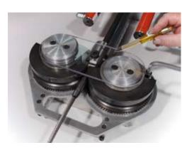
4 Move the transparent protective shield into position. Apply hydraulic pressure to draw the terminal between the roller dies.
