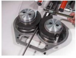
**6** Measure the diameter of the terminal after swaging, and compare with the swage dimensions list.
