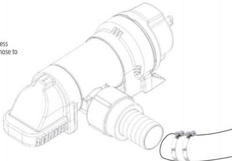
During the winterization of a vessel, it's recommended that you remove the check valve (if equipped) and drain any residual water from the plumbing.
